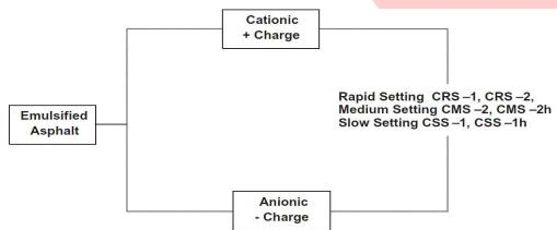
BY CHOICE OF EMULSIFYING AGENT, THE EMULSIIFED ASPHALT MAY BE: (1) ANIONIC - BINDER GLOBULES ARE ELECTRO-NEGATIVELY CHARGED. (2) CATIONIC - BINDER GLOBULES ARE ELECTRO-POSITIVELY CHARGED.ALSO, BY VARIATION IN MATERIALS AND MANUFACTURE EMULSIIFED ASPHALTS OF BOTH ANIONIC AND CATIONIC TYPES ARE MADE IN SEVERAL GRADES. SOME OF THESE GRADES AND THEIR USES ARE: (1) ANIONIC - NON -VIRGINIA GRADES RS-2
