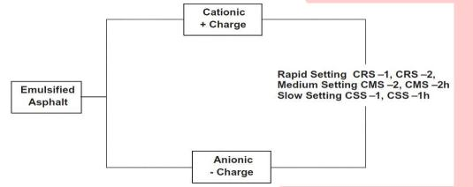
BY CHOICE OF EMULSIFYING AGENT, THE EMULSIIFED ASPHALT MAY BE: (1) ANIONIC - BINDER GLOBULES ARE ELECTRO-NEGATIVELY CHARGED. (2) CATIONIC - BINDER GLOBULES ARE ELECTRO-POSITIVELY CHARGED.ALSO, BY VARIATION IN MATERIALS AND MANUFACTURE EMULSIIFED ASPHALTS OF BOTH ANIONIC AND CATIONIC TYPES ARE MADE IN SEVERAL GRADES. SOME OF THESE GRADES AND THEIR USES ARE: (1) ANIONIC - NON -VIRGINIA GRADES RS-2
